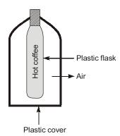
Hot coffee is separated from its cooler surroundings by a plastic flask, an air space, and a plastic cover. So all modes of heat transfer.
